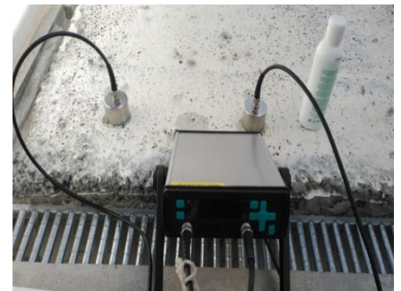
Mechanical strength measured by ultrasonic pulses
